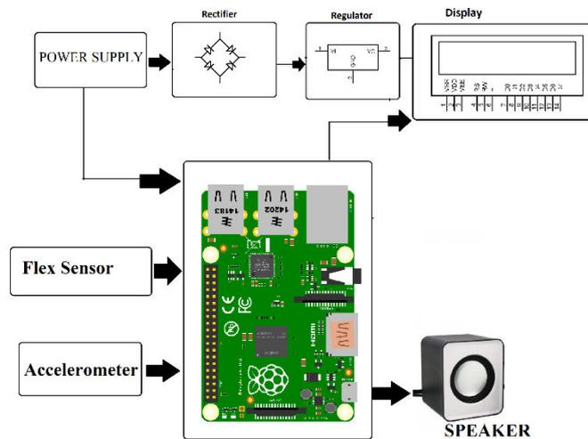
( Fig 6 Block diagram of assembled system )
